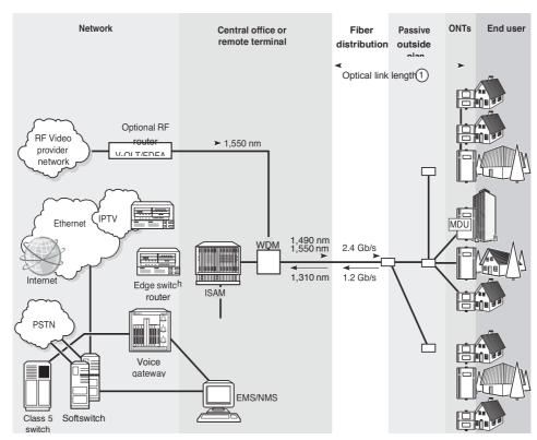
1 The maximum optical link length depends on the specific equipment and deployment conditions
